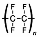
In PTFE, due to large fluorine Atom, PTFE Molecule takes up a twisted zigzag, with the fluorine atoms packing tightly in a spiral around the Carbon-carbon skeleton. This compact interlocking of fluorine atoms lead to a PTFE molecule of great stiffness leading ultimately high crystalline melting point @ 327<sup>o</sup>C, thermal stability & electrical insulation properties. Due to strong & stable bond between carbon & fluorine atom, PTFE molecule processes outstanding chemical inertness
